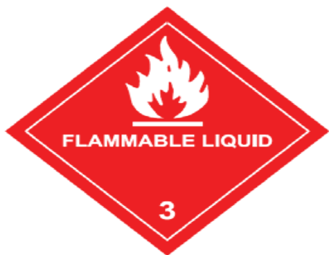
Fig 1 A universal transportation placard to be placed on trucks and drums containing flammable liquid such as hexane (sign background color is red)
